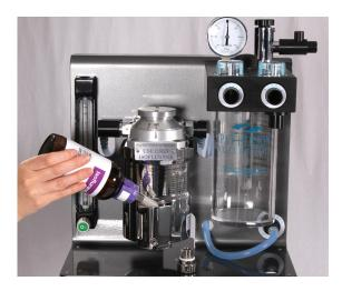
**STEP 12** Replace funnel fill cap on vaporizer after the fill operation has been completed. Tighten securely by hand.
