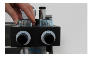
**STEP 2** Clean dome cap O-rings and all internal/external features with a mild soapy water solution, rinse well with water and dry before reinstalling. (O-ring Replacement: 07-8910887)
