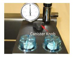
**STEP 4** Check inhalation/exhalation flutter disks. During shipping these disks MAY have come dislodged from their normal positions. They should be oriented flat on top of the valves beneath the dome caps as shown in the photo. If they are not as shown remove the dome caps, place the disks flat on the valves and replace the dome caps BEFORE using the anesthesia machine.
