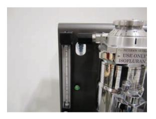
Install female endcap onto the inlet side of vaporizer manifold. Move vaporizer so that the tubing is centered with the slot as shown.
