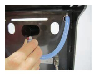
Push female endcap through large slot next to the flowmeter. Female endcap should now be positioned on the other side of frame as shown in the next picture.
