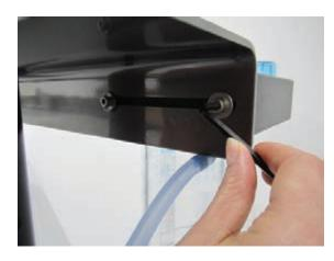
Remove both 1/4–20 socket head cap screws securing absorber block to the frame.
