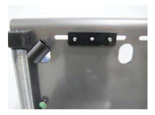
Spacer plate should now have both screws installed and centered as shown.
