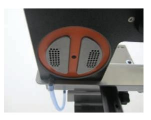
Remove absorber canister and wipe gasket clean with isopropyl alcohol. Examine holes for any blockage from CO<sub>2</sub> absorbent. (Absorber Gasket Replacement: 07-8909066)
