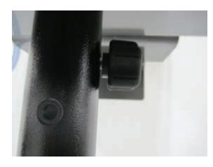
Remove pole knob and lift the head of the anesthesia machine off of pole and place it on a table or countertop.
