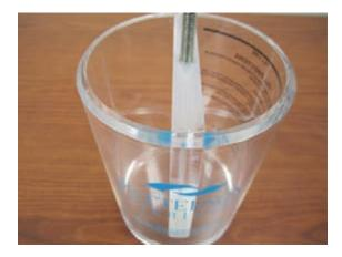
Remove all CO<sub>2</sub> absorbent and remove as much dust as possible. Clean internal/external and divider sections of absorber canister with a mild soapy water solution. Pay specific attention to the top of canister where soda sorb can build up.
