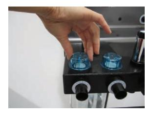
Remove dome caps as shown. (Dome Cap Replacement: 07-8910270)
