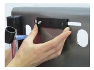
Place flat washers on M6 X 22mm screws and install through the back of frame and through spacer plate as shown.
