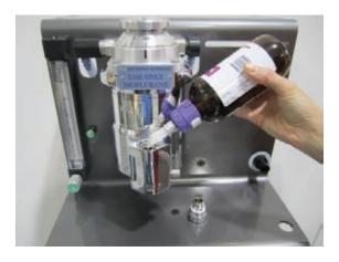
Fill vaporizer with the appropriately labeled anesthetic agent. EX III capacity is 250ml. Allow vaporizer to sit for 1 hour upon initial fill prior to use so that the wick can absorb the agent. Reference vaporizer operations manual.
