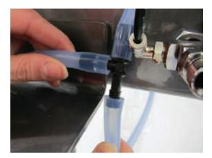
On the back of the machine, disconnect silicone tubing connected from the absorber block to the T-piece as shown.
