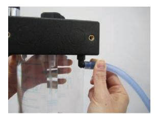
Turn elbow connector 90° clockwise (as viewed from bottom of absorber block). Hose barb will point <u>away</u> from absorber canister.
