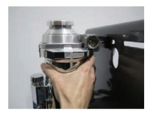
Lift vaporizer and thread screws into the vaporizer manifold. Hand tighten only at this point.
