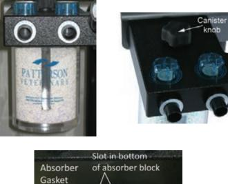
Slot in bottom of absorber block asket Canister Divider Fill absorber canister with CO<sub>2</sub> absorbent to the designated fill line and secure to anesthesia machine (with Patterson logo facing the front of the anesthesia machine) with the knob from the hardware bag.
